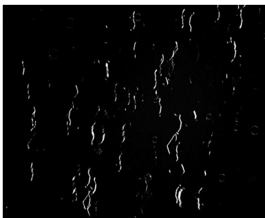
Figure 5. Microphoto of nano-composite layer (NC-2, LC matrix is ZhK1289, surfactant CTAB) in the cell with the liquid crystal layer thickness 1.8 μm treated for planar alignment. Cell was filled by capillary method at the temperature higher than the clearing point. Photo was done between crossed polarizers at room temperature. The size is 500 μm × 400 μm.
