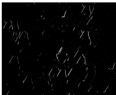
Figure 7. Microphoto of nano-composite layer (NC-4, LC matrix is 5-CB, ligand – mPEG-SH). All other conditions are the same as in the Figure 2.
