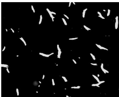
Figure 3. Microphoto of NC-1 droplet squeezed between two glasses without any aligning layers, made with crossed polarizers at room temperature. The size is 500\text{ }\mu\text{m} \times 400\text{ }\mu\text{m} .
